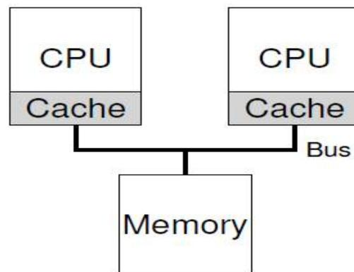
Figure 10.2: Two CPUs With Caches Sharing Memory
