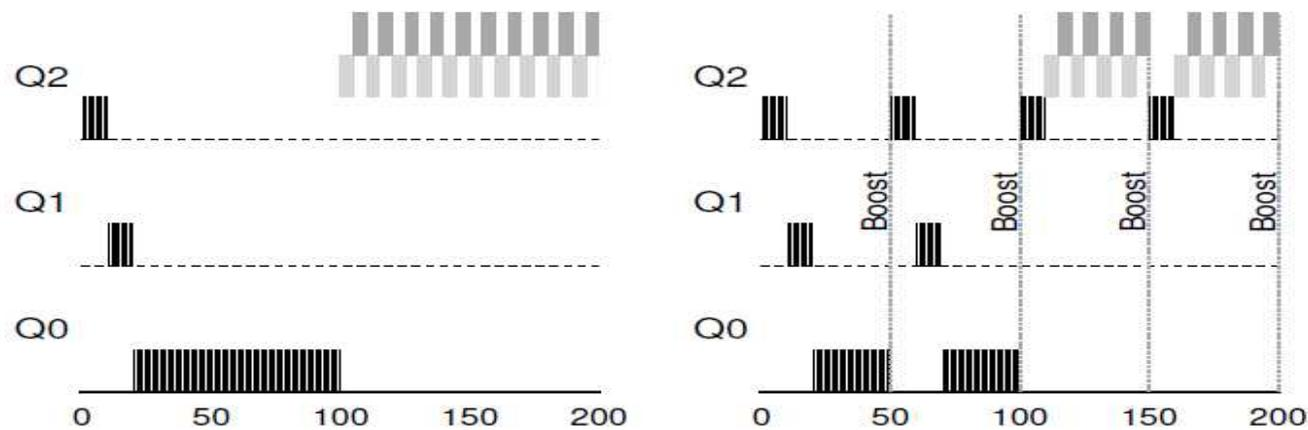
Figure 8.5: Without (Left) and With (Right) Priority Boost
