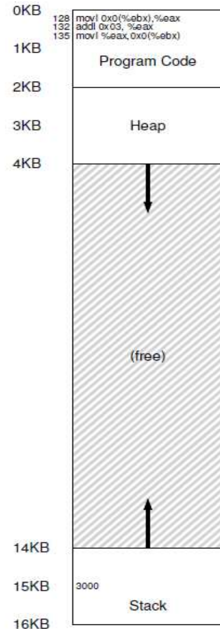
Figure 15.1: A Process And Its Address Spa
